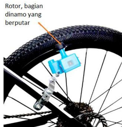
**Gambar 29.** Dinamo Sepeda
